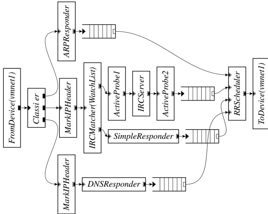
**Figure 30:** Click configuration for BotProbe. The figure shows a configuration for black-box testing on existing bot binaries. If BotProbe is deployed as a middlebox into a real network, we can remove the IRC Server, SimpleResponder, and DNSResponder elements.
