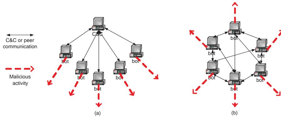
**Figure 19:** Possible C&C structures of a botnet: (a) centralized; (b) peer-to-peer.
