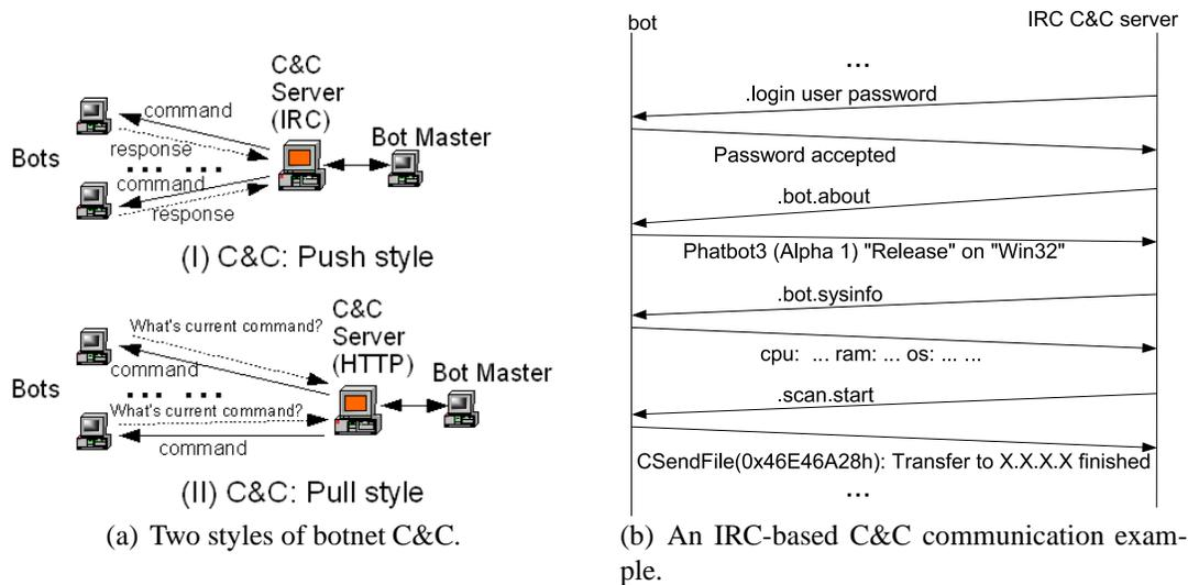
**Figure 13:** Centralized botnet command and control: two representative styles and an IRC-based example.
