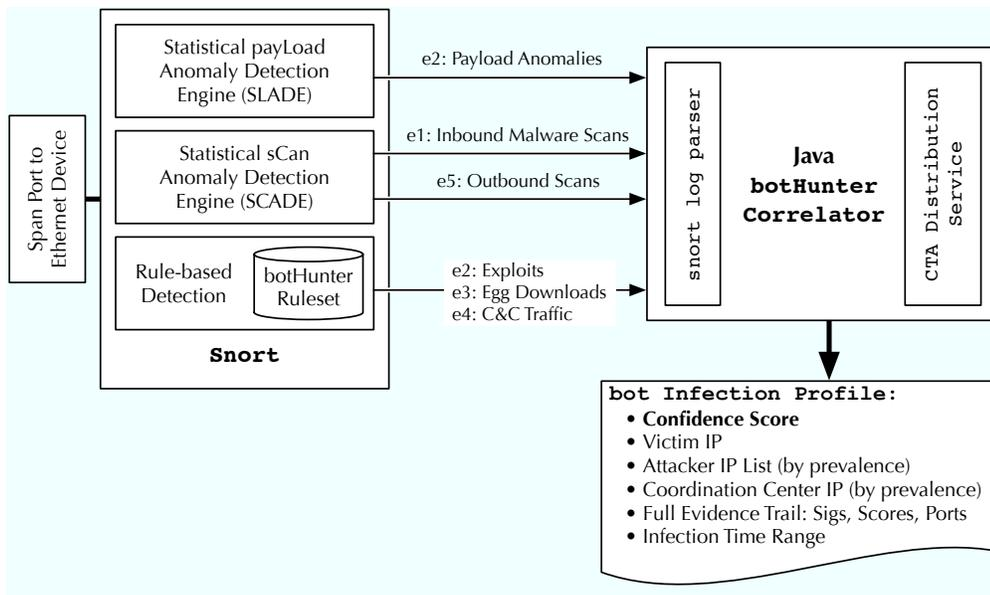
**Figure 6:** BotHunter system architecture.
