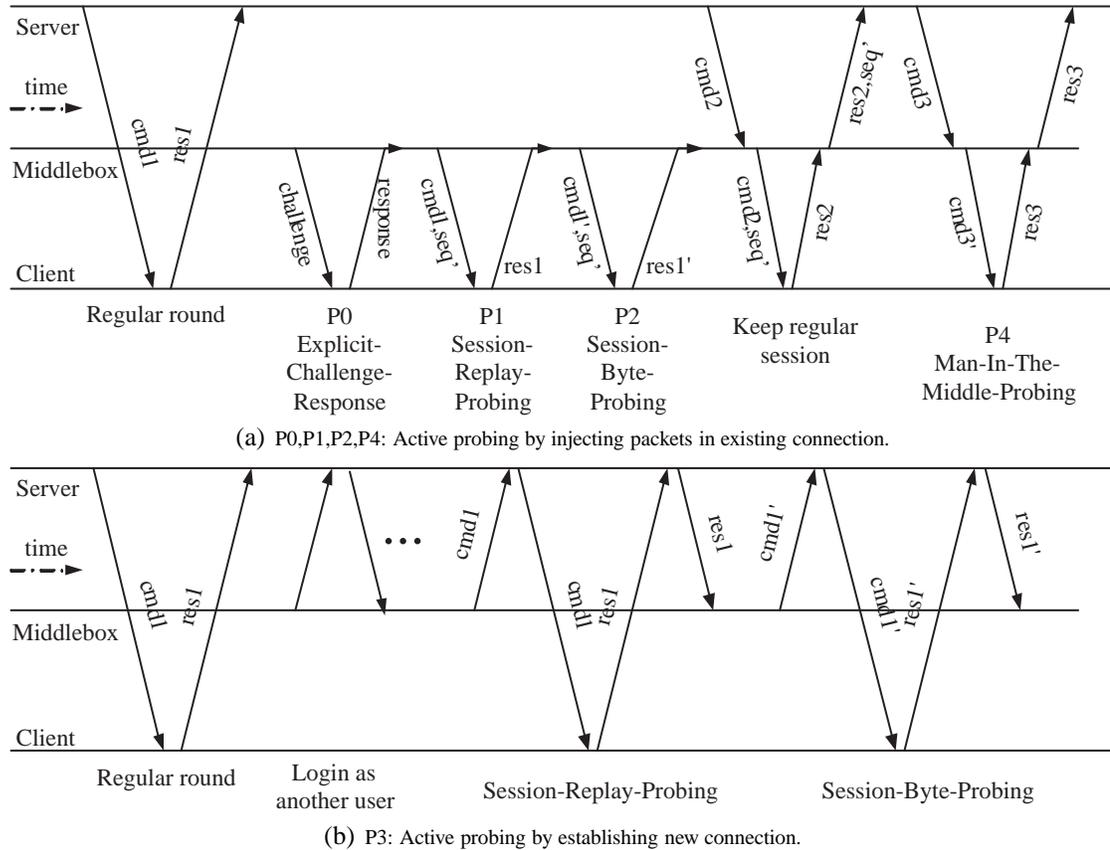
**Figure 28:** Example active probing techniques. Here *cmd'* means a modified command packet, *seq'* means modification is needed on the sequence/acknowledge number to keep the TCP session.
