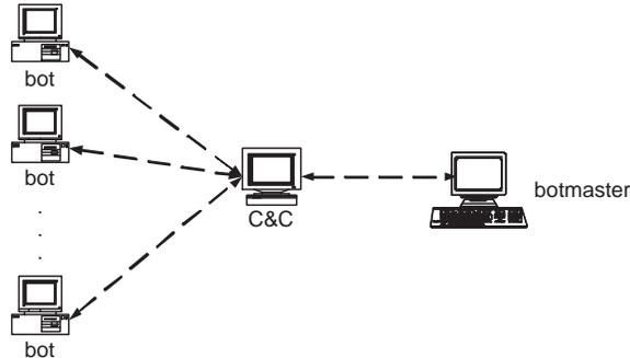
**Figure 1:** Botnet: a typical structure.
