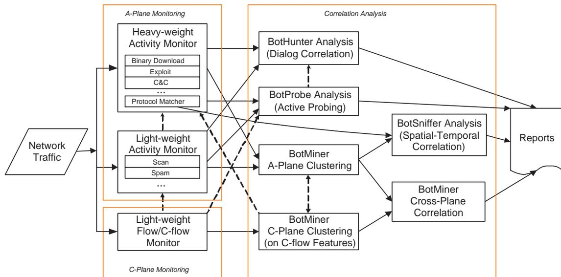
**Figure 31:** Example combination of multiple techniques in a future botnet detection system.
