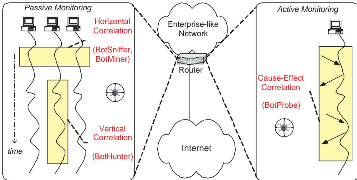
**Figure 2:** Our correlation-based botnet detection framework.
