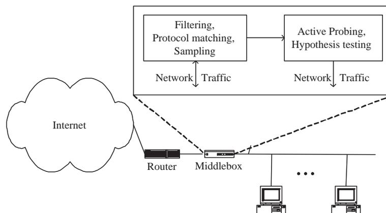
**Figure 27:** Two-layer architecture of using active techniques for identifying botnet C&Cs.
